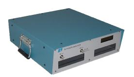
The 1040L Amplifier is a rugged source of RF power for ultrasonics, induction heating and laser modulation as well as plasma applications. It is a totally solid state solution employing RF DMoS FETs in the power amplification stages, offering simultaneous forward and reverse power readouts, and RS232 port for data collection. The 1040L reflects E&I's commitment to reliable and robust RF power.
