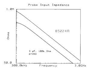
Probe with less error due to higher input impedance. For example, in a 50 ohm system at 500 MHz, the 85024A presents 455 ohms which produces a 10% signal loss from loading effects, while a 3 pF, 100 k $\Omega$  probe presents 106 ohms causing a 32% signal loss.
