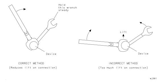
4. Hold the torque wrench lightly, at the end of the handle only (beyond the groove). See Figure 3-5.
