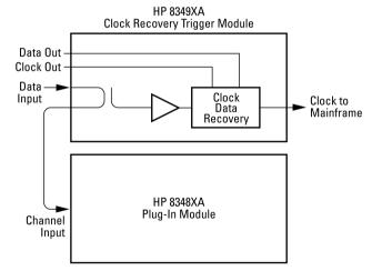
Time-domain measurements are only as accurate as the clock source that you are triggering on. All three modules have exceptional jitter performance to ensure an accurate display of jitter on the incoming data. The high sensitivity/wide bandwidth receivers also provide electrical recovered clock and electrical data regeneration for simultaneous testing with other instruments, such as the HP 71603B or 71612B error performance analyzers.
