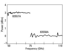
Typical maximum leveled output power for V and W band mm-wave source modules
