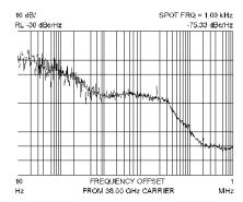
Use the 85671A phase noise utility to easily characterize noise sidebands of an oscillator.
