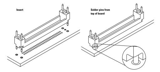
Figure 8.1. "Top-side" mountable retention module.
