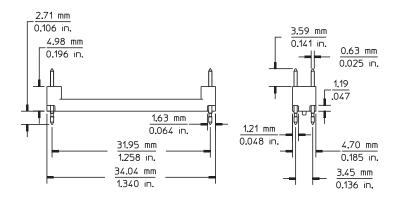
Figure 8.5. Pro Series soft touch retention module dimensions
