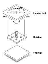
Figure 3.1. Locator tool aligning retainer on the device
