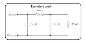
Figure 5.19. E5346A input equivalent load
