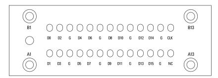
Figure 5.13. Pinout
