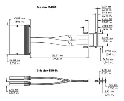
Figure 8.4. E5406A probe dimensions
