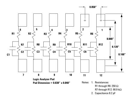
Figure 7.7. Recommended PC board pattern for 5062-7396 surface mount isolation network
