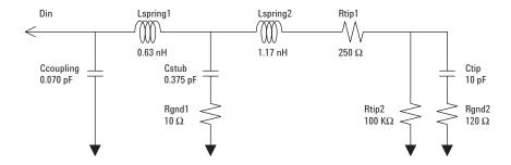
Figure 5.15. Complex (includes capacitive coupling between channels and inductance of spring pins)
