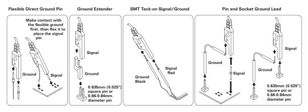
Figure 12.6. Probing configurations that give the best signal fidelity
