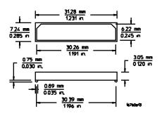
Figure 10.2. Dimensions of the 100-Pin Samtec connector used in the 16760-68702 and 16760-68703 connector kits
