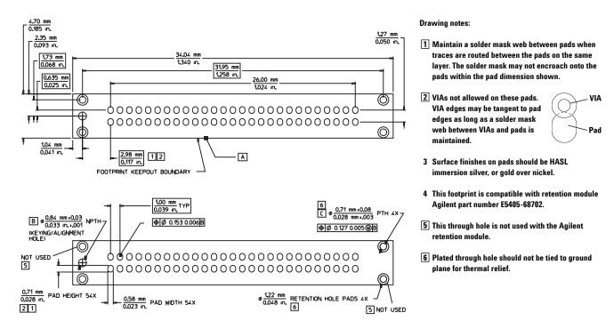
Figure 8.7. Pro Series soft touch footprint dimensions (see drawing notes).
