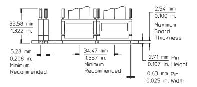
Figure 5.5. Pro Series soft touch side-by-side dimensions
