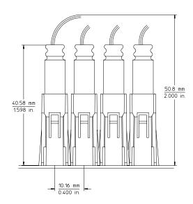
Figure 5.27. Mechanical information for E5346-44701, E5346-44703, E5346-44704 support shrouds for 38-pin Mictor connectors
