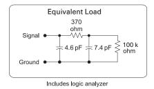
Figure 7.3. Isolation adapter (01650-63203) and equivalent load
