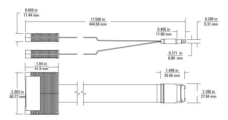
Figure 5.17. E5346A, E5351A, E5339A mechanical dimensions
