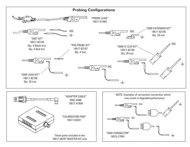
Figure 12.5. Agilent Technologies 16517-68701 master accessory kit and 16518-68701 expansion accessory kit
