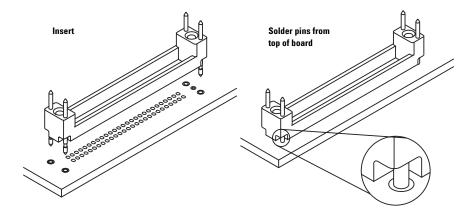
Figure 5.1. "Top-side" mountable retention module.
