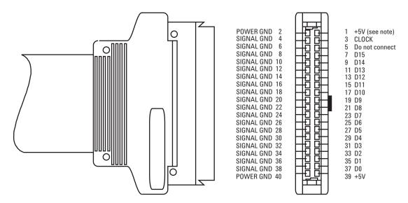
Figure 7.4. Pinout for probe cable
