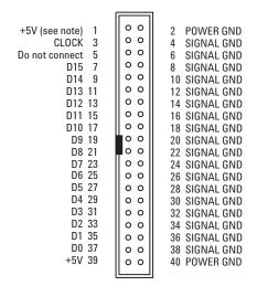
Figure 7.6. Forty-pin connector pinout
