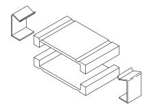
Figure 2.3. Ferrite core assembly, 16555-60001
