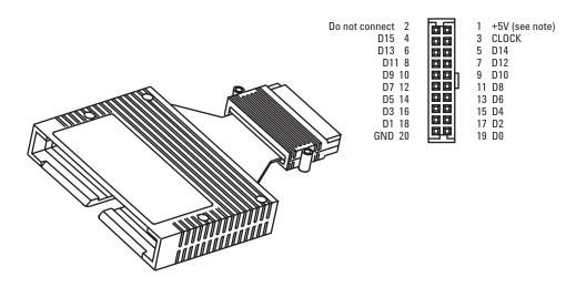
Figure 7.5. Pinout for 100 k $\Omega$  isolation adapter (Agilent part number 01650-63203)
