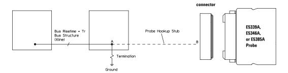
Figure 5.22. Agilent E5339A, E5346A, and E5385A design rules
