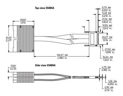
Figure 5.3. E5404A probe dimensions
