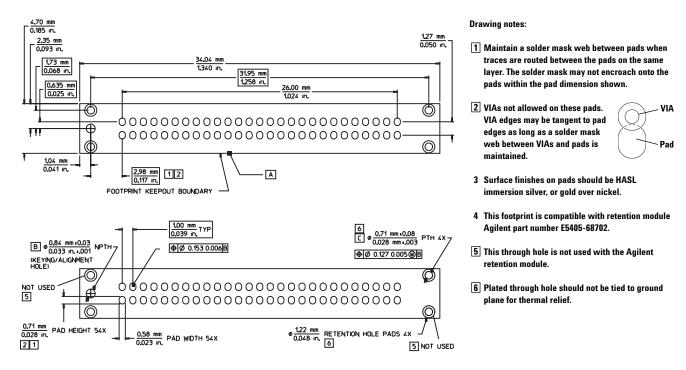
Figure 5.9. Pro Series soft touch footprint dimensions (see drawing notes).
