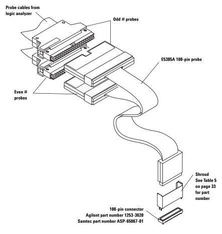
Figure 5.23. Agilent E5385A connection and pinout
