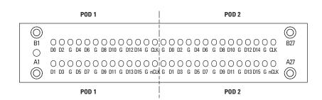
Figure 8.16. Pinout
