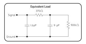
Figure 5.20. E5385A input equivalent load
