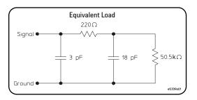
Figure 5.18. E5339A input equivalent load
