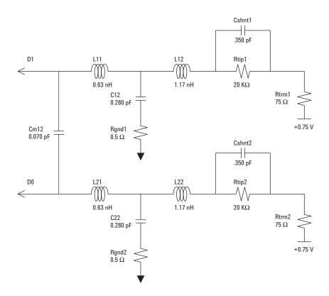
Figure 8.17. Equivalent probe load model
