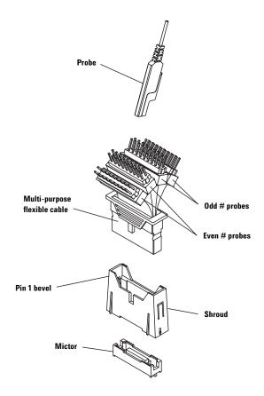
Figure 6.1. E5346-60002 Mictor break-out adapter
