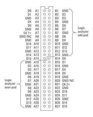
Figure 8.8. Pad numbers for E5404/06A 34-channel single-ended probes.
