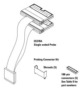
Figure 8.18. Agilent E5378A probe
