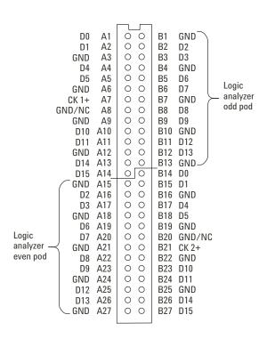
Figure 5.10. Pad numbers for E5404/06A 34-channel single-ended probes.
