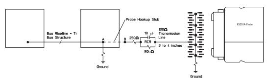
Figure 5.24. Agilent Technologies E5351A design rules
