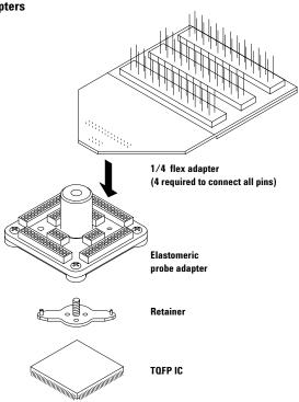
Figure 3.2. Elastomeric probing solution
