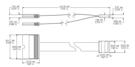
Figure 5.16. E5385A 100-pin probe mechanical dimensions
