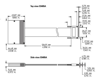
Figure 8.3. E5405A probe dimensions
