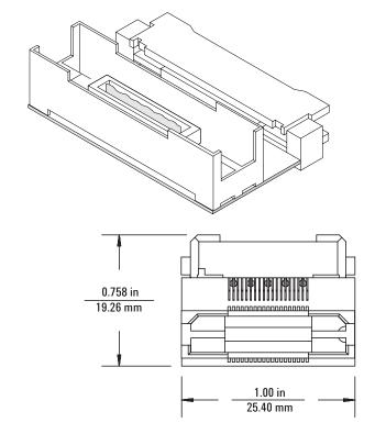
Figure 7.1. E5346-63201 right-angle 38-pin adapter
