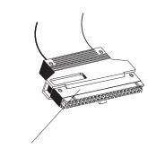
Figure 1.1. 40-pin pod connector
