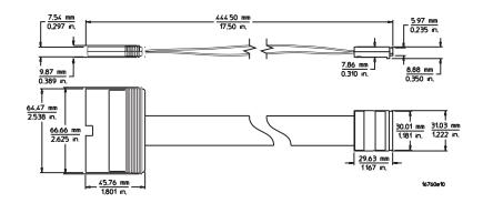
Figure 10.3. E5378A 100-pin single-ended probe dimensions
