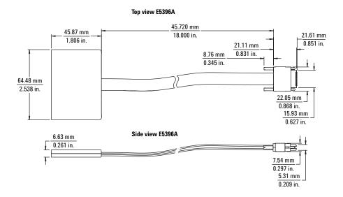
Figure 5.6. E5394A and E5396A soft touch probe dimensions
