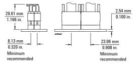
Figure 5.8. Side-by-side dimensions
