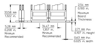
Figure 8.6. Pro Series soft touch side-by-side dimensions
