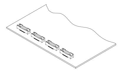
Figure 7.2. 38-pin connectors placed for use of right-angle adapter
