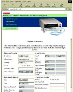
receives data over the network. It also reads and sets network parameters.
