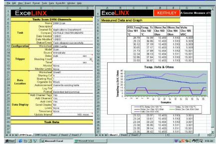
ExceLINX-1A is an economical, easy-to-use add-in utility for Microsoft<sup>®</sup> Excel and Integra systems. No programming is required; enter values quickly through pop-up menus and eliminate time-consuming coding.
