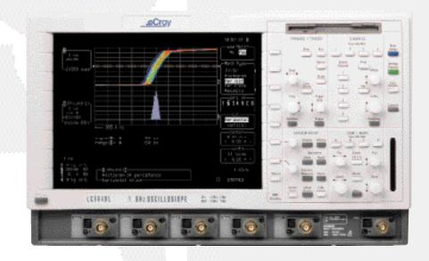
The LC564DL and LC554DL digital oscilloscopes from LeCroy are designed to save engineers valuable time in troubleshooting and problem solving. Each oscilloscope is an integrated and powerful system providing the capability to:
