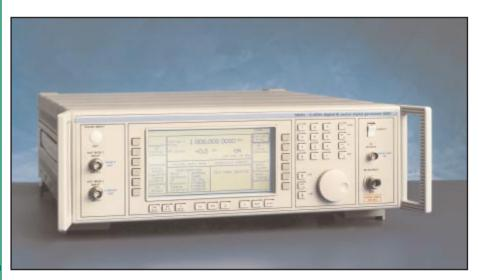
Two FM modes are available, wideband FM (>10 MHz) for fast FSK or video applications and a 1 MHz bandwidth mode. Both modes offer FM deviations up to 1% of carrier frequency. FM is available as either DC or AC coupled. A patented FM nulling correction system eliminates carrier frequency offsets that occur with lesser generators when using DCFM, and allows the 2050 to be used confidently with Wireless LAN or paging equipment such as POCSAG, FLEX™ and ERMES.
