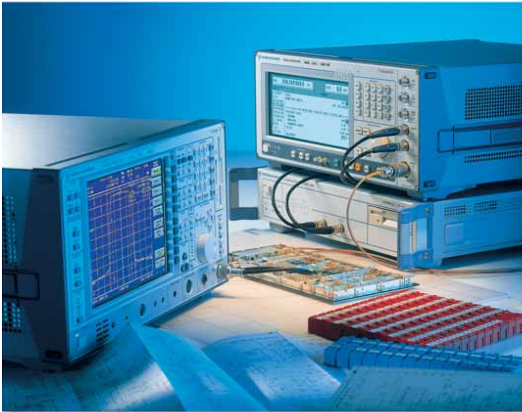
Module test with R&S SMIQ, R&S AMIQ and Signal Analyzer R&S FSIQ
