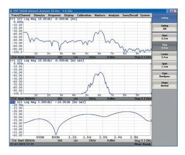
This function mathematically removes unwanted responses in the time domain, which allows the user to obtain frequency response without influence from fixture elements.
