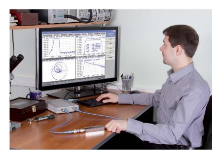
The 5048 VNA is an S-parameter vector network analyzer designed for operation with an external PC. It connects to any Windows-based computer via USB and delivers accurate testing and measurement through a platform that can keep up with constant advancements as well as be remotely accessed.
