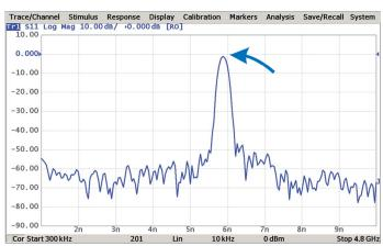
This function performs data transformation from frequency domain into response of the DUT to various stimulus types in time domain. Modeled stimulus types: bandpass, lowpass impulse, and lowpass step. Time domain span is set by the user arbitrarily from zero to maximum, which is determined by the frequency step. Windows of various forms are used for better tradeoff between resolution and level of spurious sidelobes.
