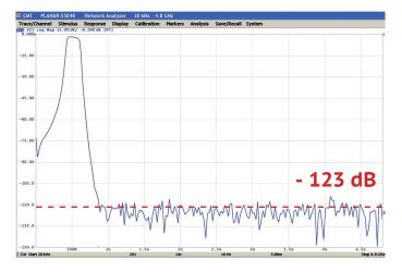
Typical dynamic range of 123 dB is achieved through the entire frequency range (at 10 Hz IF bandwidth). Seen here is the maximum dynamic range achieved when using IFBW 10 Hz and an output power level of 5 dBm.
