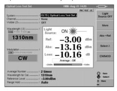
\* Light source function is mounted on MW9076B/C as standard. Power meter function is optional to MW9076B/B1/C.
