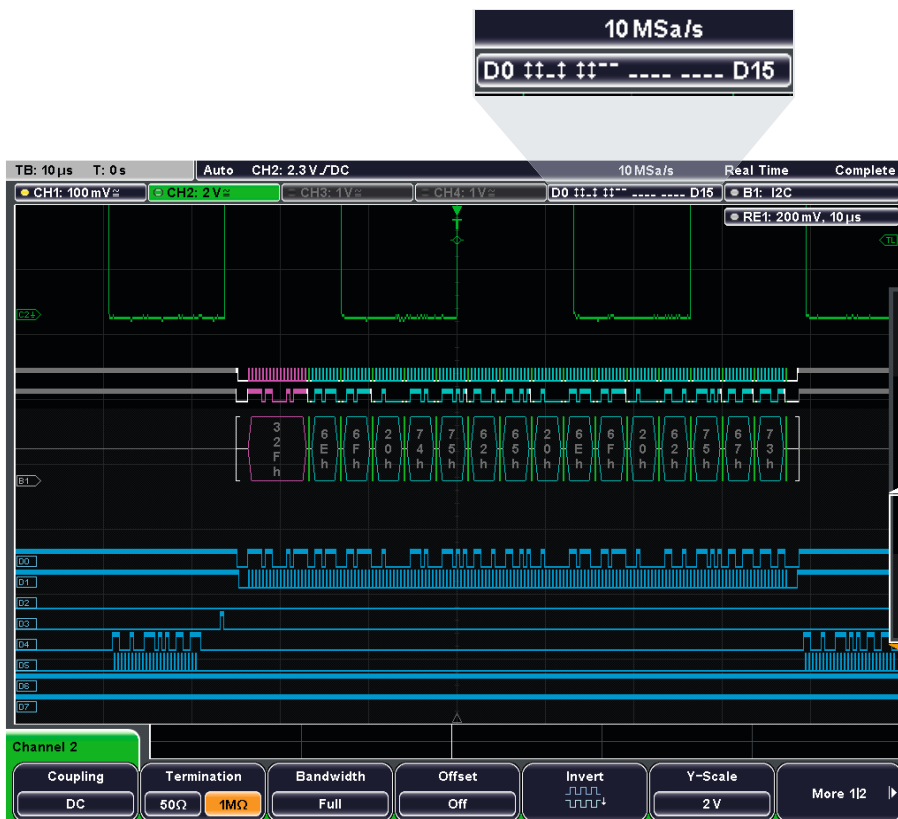
Activity display: status information for the digital signals independent from acquisition and instrument settings.
