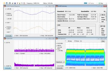
Analysis options for 802.11 standards are available. Here, an 802.11ac 160 MHz bandwidth signal is analyzed, with displays of EVM vs. subcarrier number and symbol number, channel response vs subcarrier with a summary of WLAN measurements, and the DPX spectrum of the analyzed signal. An EVM of -44.26 dB and other signal measurements are seen in the summary panel.
