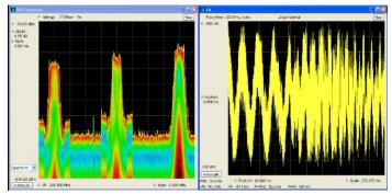
Audio monitoring and modulation measurements simultaneously can make spectrum management an easier, faster task. Here, the DPX spectrum display shows a live spectrum of the signal of interest and simultaneously provides demodulated audio to the internal instrument loudspeaker. FM deviation measurements are seen in the right side of the display for the same signal.
