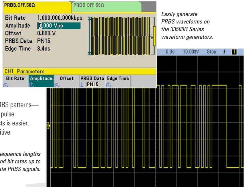
*Easily generate PRBS waveforms on the 33500B Series waveform generators.*
