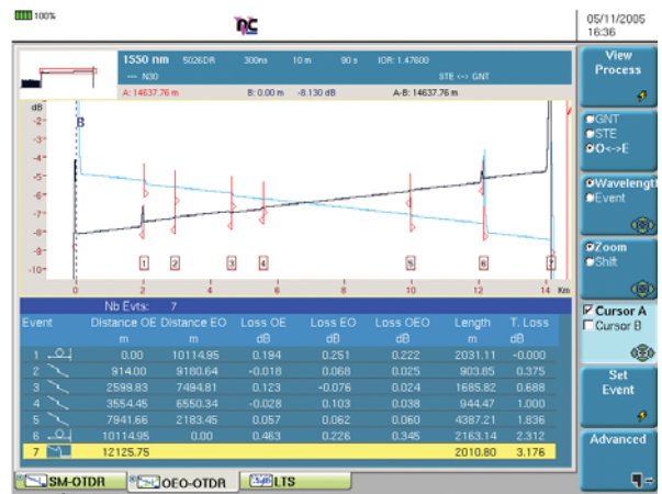
Automatic Bi-directional OTDR Analysis
