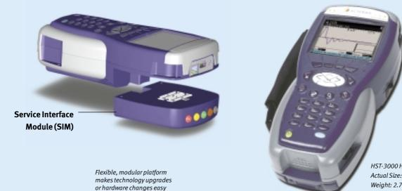
HST-3000 Handheld Services Tester Actual Size: 9.5 x 4.5 x 2.75 in Weight: 2.7 lb with battery
