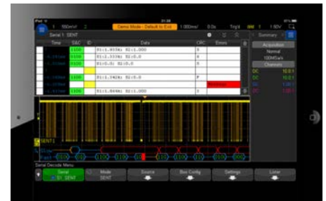
Figure 8. Remotely control the 3000T X-Series via tablet device.
