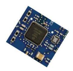
S-Series front-end includes three new custom ICs including a 130 nm BiiCMOS IC that incorporates user-selectable analog filters and bandwidth upgrades via a software license.
