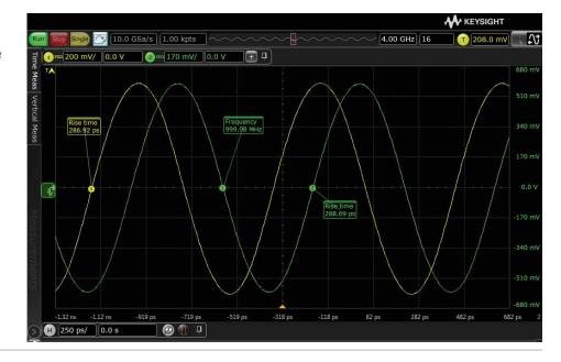
Noise directly impacts vertical placement of each signal point. Oscillocopes with lower noise have more accurate vertical placement. S-Series oscilloscopes incorporate next-generation technology to deliver the lowest noise measurements in the industry. Here's a compare at 4 GHz with 5 mV/div scaling.
