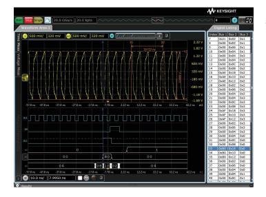
Use the digital channels to evaluate control signal relationships and data buses up to 16 bits wide. Use symbols to quickly interpret waveforms.
