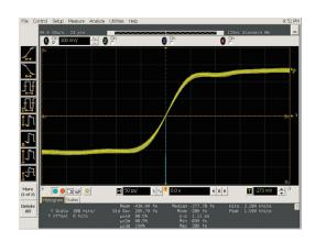
The industry's lowest trigger jitter, less than 500 fs (rms) (typically, less than 200 fs (rms) on 5 Gbps PRBS signal), facilitates accurate waveform viewing of multiple waveforms.
