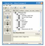
The Agilent N5392A Ethernet Electrical Performance Validation and Ccompliance Software performs a wide range of electrical tests to meet the Ethernet electrical specifications for 1000Base-T, 100Base-TX and 10Base-T systems as documented in the IEEE 802.3-2005 and ANSI X3.263-1995 standards.
