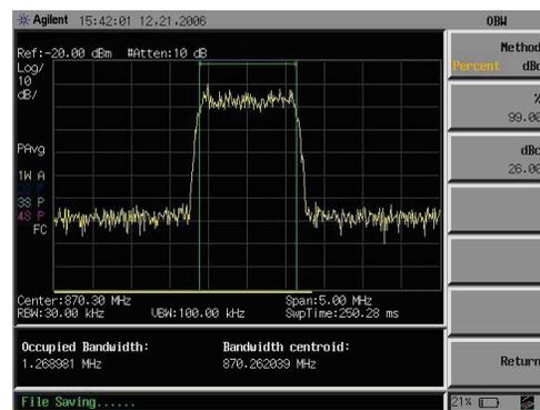
The occupied bandwidth is measured in percentage.
