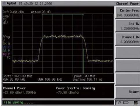
It is quick and easy to set center frequency, integration bandwidth, and channel bandwidth on the panel.
