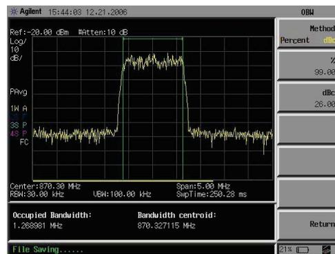
The occupied bandwidth is measured in dBc.
