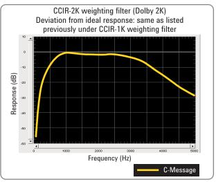
Figure 15. CCIR-2K weighting filter
