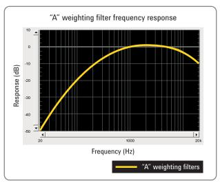
Figure 14. "A" weighting filter frequency response
