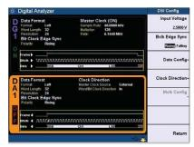
Figure 1: Configure your digital generator DSI settings, including the output format of your choice. Choose amongst four formats: I<sup>2</sup>S, Left Justified, Right Justified
