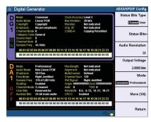
Figure 2: The general AES3/SPDIF output settings can be configured with the status bit type, status bits, audio resolution and output voltage, with mode settings set to either "Consumer" or "Professional."
