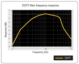
Figure 17. CCITT filter frequency response
