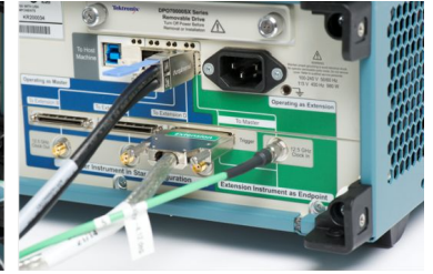
UltraSync connection on instrument with Extension role
