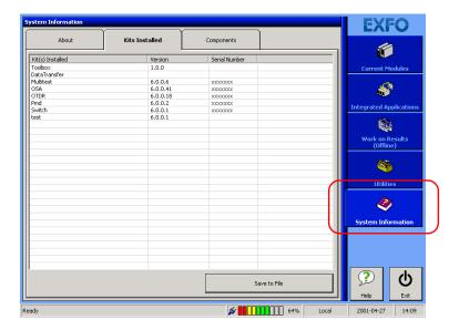
2. Select Kits Installed to view which kits are installed on your unit.
