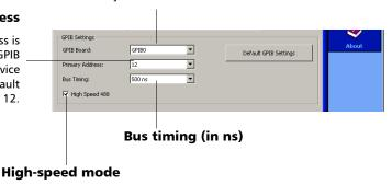
Check the box to enable high-speed mode.
