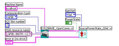
**9.** Repeat steps 7 and 8 for each of the functions you want to use. However, except that you have to link the *Communication ID in* parameter of the new driver to the *Communication ID out* parameter of the preceeding driver.
