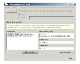
With this demo application, you can control your FTB-400 Universal Test System either in local (COM technology) or remote (DCOM technology) mode. If you want to work in remote mode, see *Preparing for Remote Control with DCOM* on page 90.
