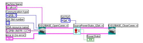
Connect the *Communication ID out* parameter of the last function to the *Communication ID in* of EXIQSBASE\_CloseComm.vi.
