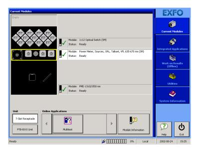
ToolBox 6 brings multitasking to field testing. You can perform different tests and work on tests results all at the same time, switching between applications simply by touching a button. You can also run applications requiring the combination of several modules by setting the combination of modules to use, and launching the application.
