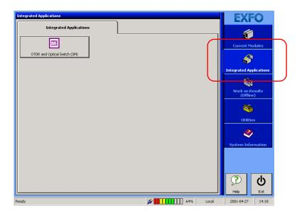
Applications will appear in the **Integrated Applications** tab only if the required modules are already inserted into the FTB-400 Universal Test System.
