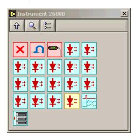
On a particular icon, the displayed symbol refers to the first keyword of the associated SCPI command. The background color is a function of the command type:
