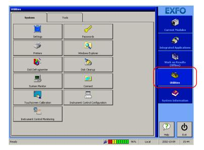
**2.** Click on **Instrument Control Monitoring** to access the corresponding utility.
