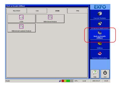
Each module has its own tab, on which you will find related applications. The applications will vary according to the modules you have installed in your unit. You do not need the module to be physically inside the FTB-400 Universal Test System, but the corresponding software must be installed.
