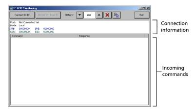
**3.** Connect to the monitoring system by clicking on **Connect to IC**. To disconnect from the monitoring system, simply click on **Disconnect from IC**.
