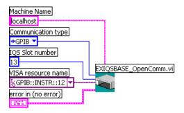
**5.** Set the communication parameters. For information on communication parameters, see *Working with EXFO LabVIEW Drivers* on page 122.
