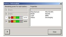
By clicking on a battery, you will see relevant details, such as the model, type and manufacturer, as well as the current status (charging or discharging).
