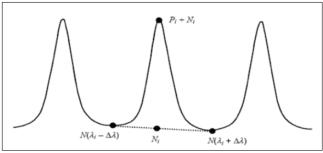
Figure 1: Interpolation method (ref.: IEC 61280-2-9 Ed.2)
