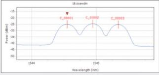
Figure 3: 40G network requiring in-band OSNR measurement.
