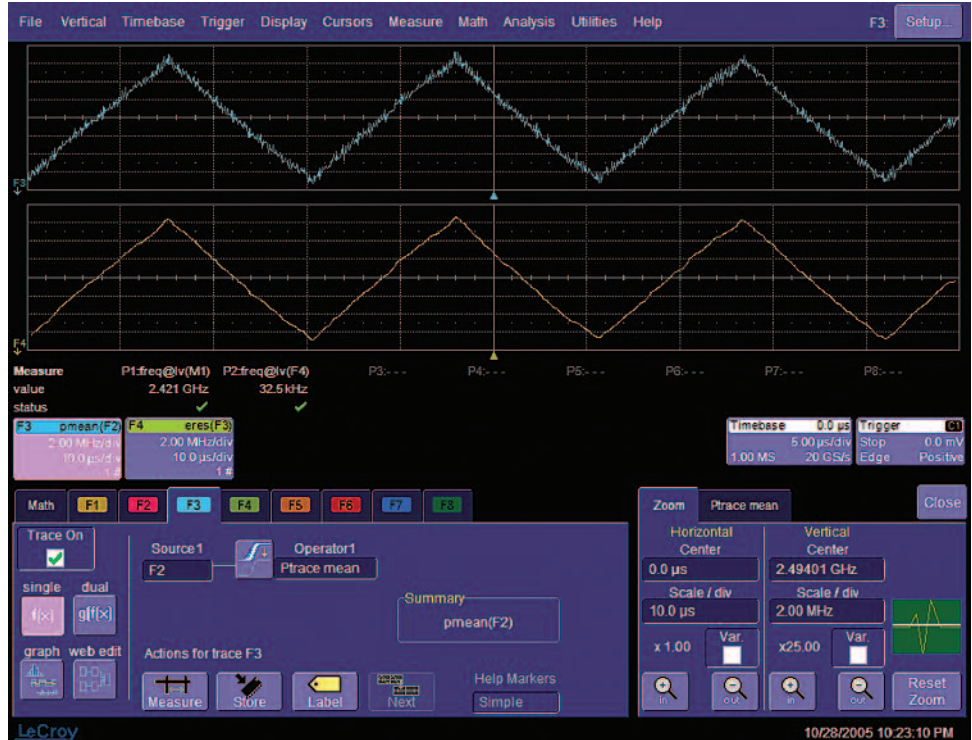
See multiple cycles of spread spectrum clocking.
