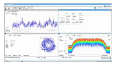
In the illustration above, a 5 GHz carrier modulated with 500 MSymbols/sec pi/4-QPSK is analyzed with the RSA7100A Option B800 and SignalVu-PC application license SVMH. A measurement summary, EVM vs. Time, and constellation display are shown along with the continuous monitoring of the DPX spectrum.
