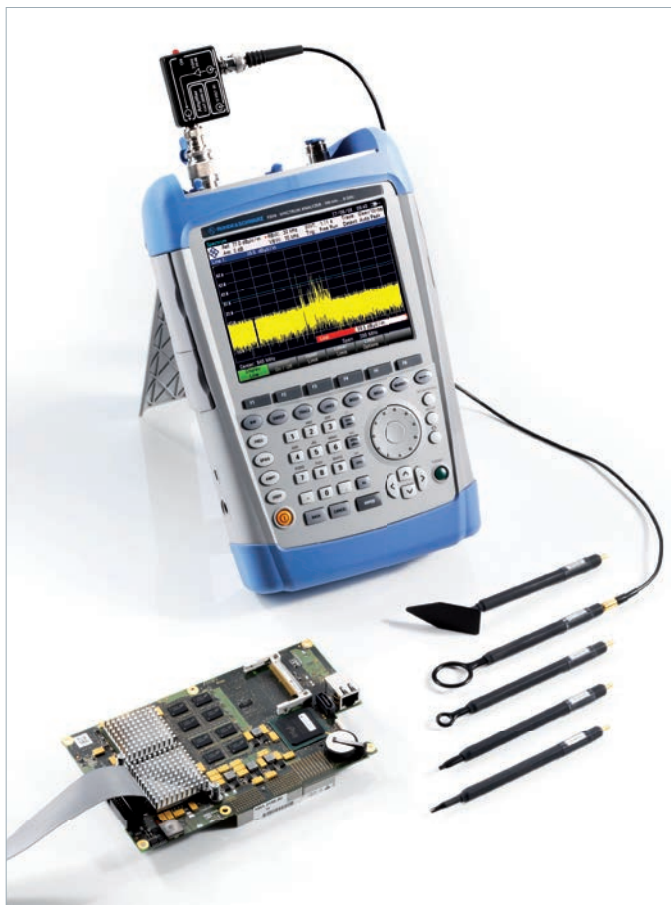
The R&S®FSH8 with near-field probes and DUT.
