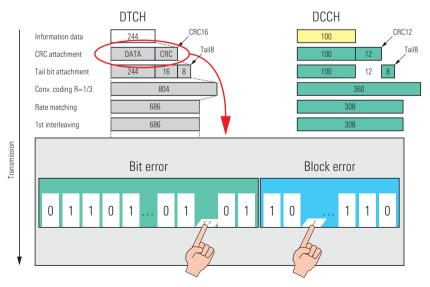
Insertion of bit errors and block errors into the output signal
