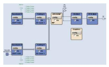
Setup for simulating transmit diversity with fading
