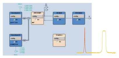
Generation of 3GPP and GSM/EDGE signals in realtime
