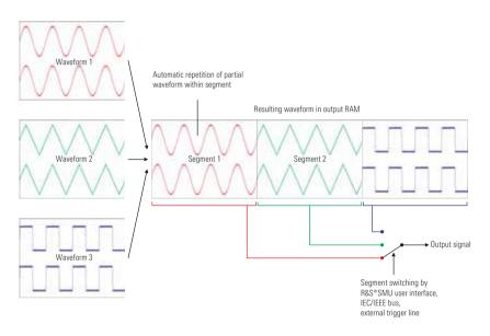
How the multisegment waveform operates
