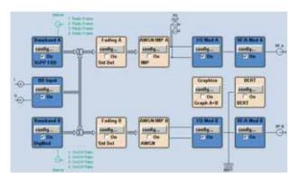
Addition of external I/O signals to internal baseband signals
