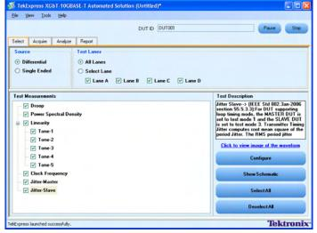
**XGbT 10GBASE-T Automated Compliance Software** – Quickly perform 10GBASE-T measurements per the IEEE 802.3an-2006 standard including Power Spectral Density (PSD), Power Level, and Linearity, with a simplified instrument configuration. XGbT provides flexible control over test configurations and analysis parameters, enabling more in-depth device characterization.
