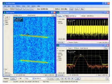
SignalVu™ Vector Signal Analysis – Easily verify wide-bandwidth designs such as wideband radar, high data-rate satellite links, or frequency-hopping radios and characterize wideband spectral events. SignalVu combines the functionality of a vector signal analyzer, a spectrum analyzer, and the powerful triggering capabilities of the DPO/DSA70000B and MSO70000 – all in a single package.
