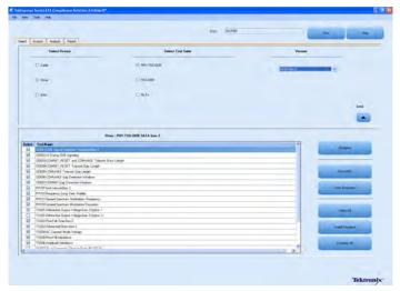
**TekExpress SATA Automated Compliance Test Software** – Complete support for SATA Gen1 and SATA Gen2 defined test suites. Reduce your compliance test time by approximately 70% with simple, efficient automation of all required test suites with TekExpress software. Also included is auto-recognition of all required test equipment, precise DUT/Host control, and one-button testing.
