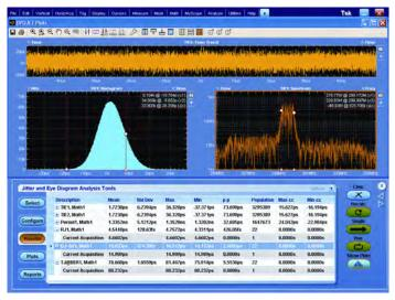
**DPOJET Jitter and Eye Diagram Analysis** – Simplify identifying signal integrity concerns, jitter, and their related sources with DPOJET software. DPOJET provides the highest sensitivity and accuracy available for real-time oscilloscopes.
