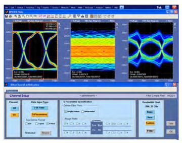
**SDLA - Serial Data Link Analysis (Option SLE and SLA)** – Offers the capability to emulate the serial data channel, de-embed a fixture or other network, and add or remove transmitter equalization. Option SLA adds processing of waveforms with FFE and DFE equalizations and automatic equalizer training. DPOJET provides advanced measurement and jitter analysis of the resulting waveforms.
