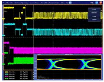
**MIPI® D-PHY Transmitter Characterization and Compliance Test Solution (Option D-PHY)** – Verify to the D-PHY specification, rapidly characterize and discover sources of jitter and signal integrity concerns. Perform high-speed data-clock timing measurements, along with other electrical characteristics in high-speed or low-power modes.
