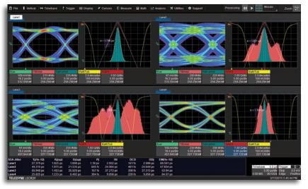
equalization schemes (using Eye Doctor II option) or examining system behaviors at different locations in the link (using probes or the VirtualProbe option).
