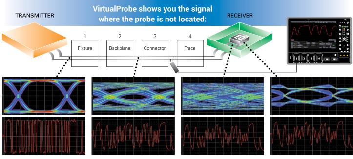
Virtually probe the signal at the transmitter with the fixture present, and then de-embed its effects form the measurement. View the signal between structures to understand losses, ISI and crosstalk caused by backplanes, interconnects and connectors.
