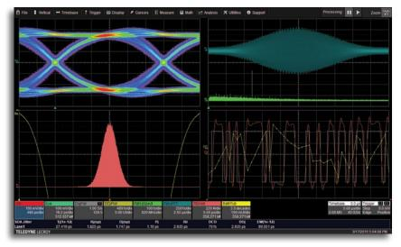
The Teledyne LeCroy SDAIII-CompleteLinQ Serial Data Analysis products include multi-lane eye and jitter analysis, LaneScape<sup>™</sup> comparison modes, vertical noise measurements, and crosstalk analysis tools. These capabilities provide the deepest insight into the behavior of multi- or single-lane serial data systems.
