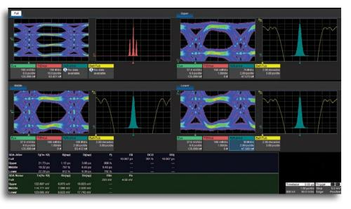
PAM4 represents a new step in the evolution of serial data signaling formats, overcoming some fundamental limitations of traditional NRZ signaling. But with new signal types come new measurement needs. Teledyne LeCroy's PAM4 analysis package meets these needs by leveraging industry-leading eye, jitter, and noise analysis capabilities to fully characterize PAM4 signals.
