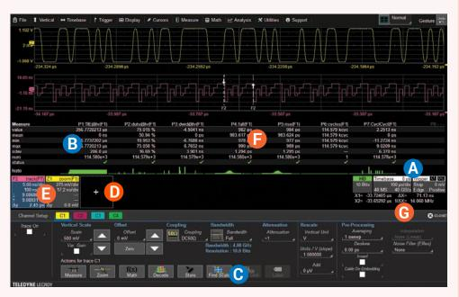
A Channel, timebase, and trigger descriptors provide easy access to controls without navigating menus.
