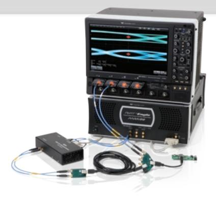
The combination of the SDA 8 Zi-A Serial Data Analyzer, the PeRT<sup>3</sup> and the SPARQ provides the most comprehensive solution for serial data compliance testing. These three pieces of equipment enable a full suite of physical layer compliance testing and debugging ability that will guarantee the best signal integrity for your serial data signals.
