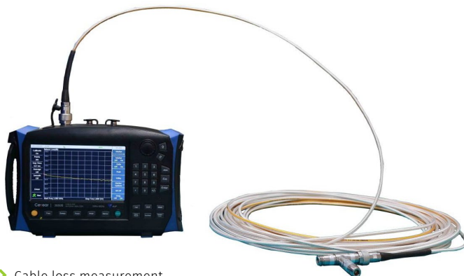
➤ Cable loss measurement
