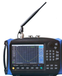
➤ Antenna return loss/VSWR measurement
