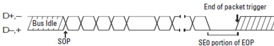
Figure 5-9 USB Data Transmission Protocol
