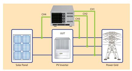
User could implement 3P3W (Three Phase Three Wire) wiring mode for three phase power measurement application. Such as Power Supplies.
