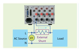
66203/66204 Power Meters support external shunt function for high current (>20A) measurement application.
