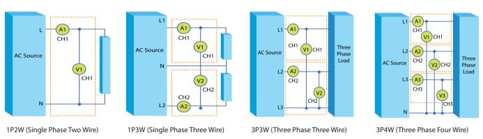
Each channel of 66203/66204 has the ability to provide independent measurements; hence the meters are suitable for multi-point measurement applications such as PV inverter testing. Instruments are designed for measuring DC input parameters as well as three phase AC readings on the output side. The overall efficiency for the PV inverter can easily be obtained by built-in functions. In order to meet high voltage applications (up to 1200Vrms) Chroma offers an HV option kit.
