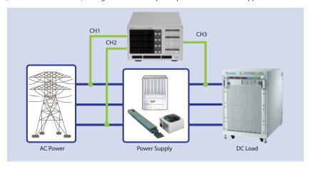
With the wiring mode set as 1P2W, the 66204 Power Meter has the capability of performing up to 4 simultaneous power measurements as shown. The meters are also designed to comply with power measurement requirements in accordance to many international standards such as Energy Star/EN 50564/IEC 62301/ ErP.
