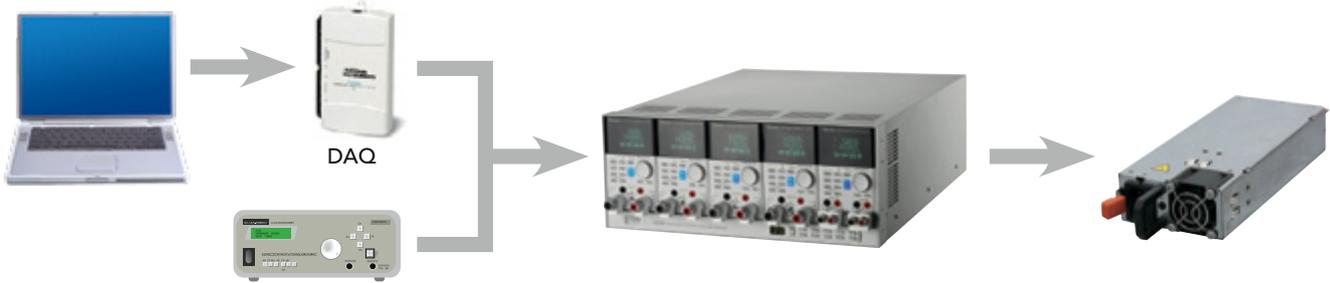
To reconstruct the actual current waveform, one can simply upload the captured waveform data into any module via a Chroma softpanel. Each module is capable of storing up to 10 sets of waveforms with each comprising up to 1.2 millions data points to meet the more strenuous test requirements.
