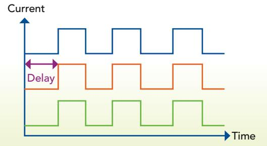
Peak power cycle test for printer power (Three output channel for UUT)
