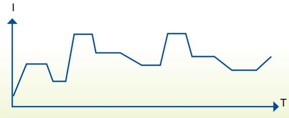
Simulations of all kinds of real current waveforms for battery discharge testing and other applications are possible. (Notebook, Electric car and Electric bike) (Single output channel for UUT)
