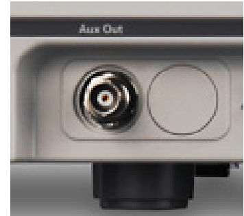
Figure 21. Aux Out is used in the calibration procedure for each channel by connecting the sensors and probe adapter. As the connection cable is included in the mainframe, you can immediately start the User Calibration.
