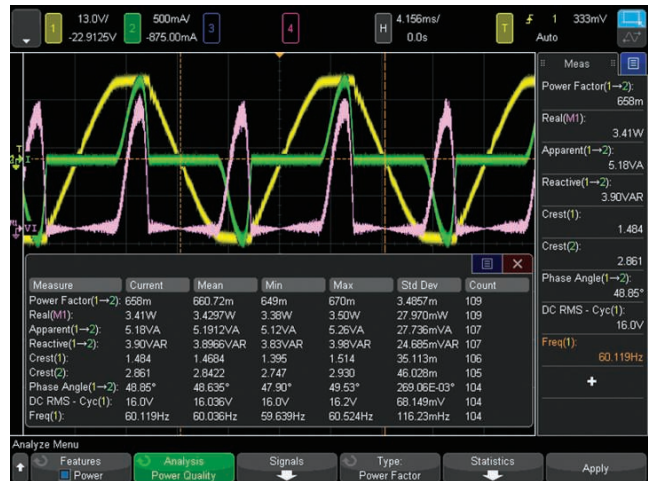
Figure 25: Power quality measurement, one of many in the power measurements application.
