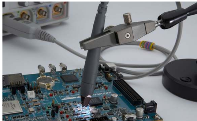
Figure 34: The N2750A InfiniiMode probe allows convenient measurement of differential, single-ended, and common mode signals with a single probe tip without reconnecting the probe to connection.
