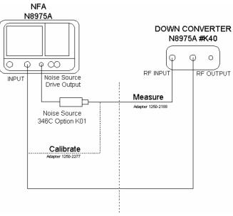
Figure 4-2 Test Set-up for LO Accuracy and Troubleshooting
