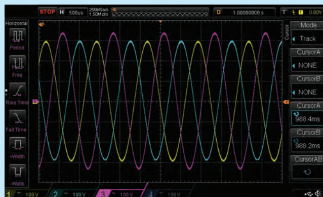
Three Phase Unbalance Voltage Test Captured
