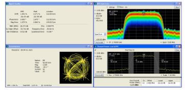
Time-correlated views in multiple domains provide a new level of insight into design problems not possible with conventional analyzers. Here, ACLR and modulation quality are performed simultaneously in a single acquisition, combined with the continuous monitoring of the DPX<sup>®</sup> spectrum display.
