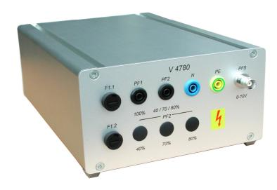
The tapped transformer can be used to simulate power supply failures as voltage interruptions. The basic standard EN/IEC 61000-4-11 Ed.2 specifies this phenomena.
