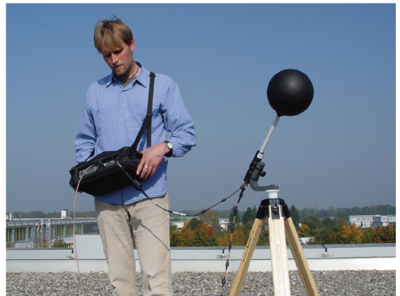
Measurement with the handheld spectrum analyzer and the 9171 Isotropic Antenna
