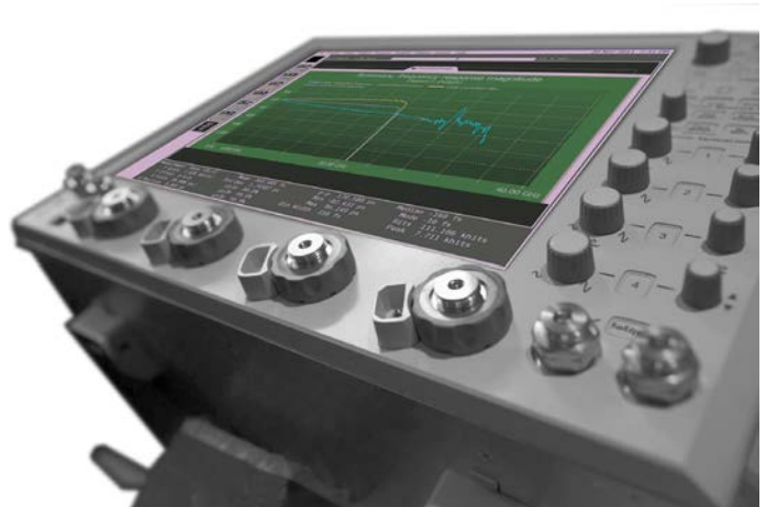
PrecisionProbe software characterizes cables to 63 GHz
