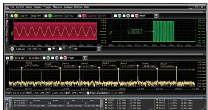
Peak search capability makes InfiniiView a frequency domain tool
