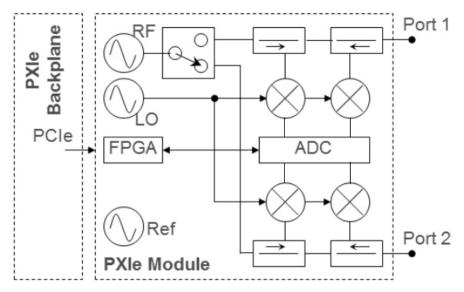
PXIe Vector Network Analyzer block diagram
