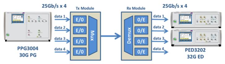
100G Ethernet four lane end-to-end test using PPG3000 series pattern generator and PED3200 series error detector
