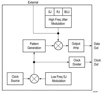
Jitter insertion block diagram
