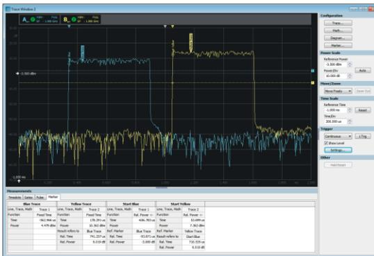
Pulse delay measurement on different traces.
