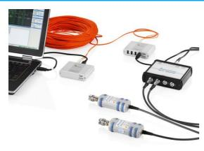
The power sensors can be operated either on an R&S\*NRP2 base unit or directly on a laptop/PC. They are also supported by numerous Rohde & Schwarz signal generators, signal analyzers, spectrum analyzers and network analyzers. The R&S\*NRP-Z4 passive USB adapter cable is all that is needed to connect the sensors to a laptop/PC.
